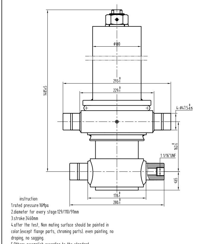
5.0thers accomplish according to the standard QC/T460-2010<<cylinder for dump truck technology>>
